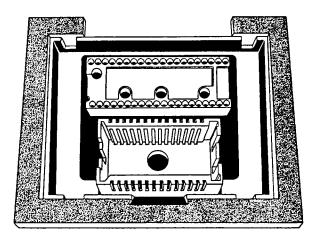
4. Align the ends of the ROM as shown here:
